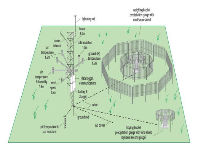
Figure 1. Proposed Typical CRN Station Configuration
